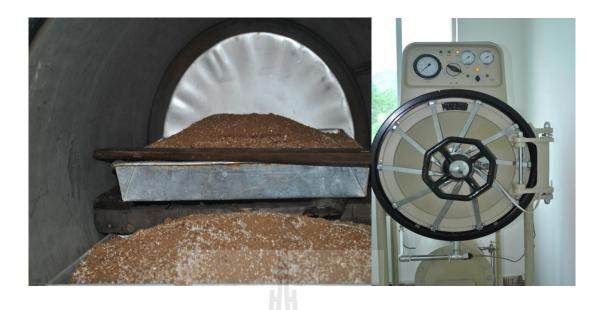
Appendix figure 1: Soil sterilization (left) and high pressure sterilizer (right)
