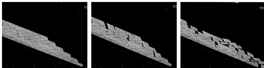
Figure 4.7 Some test results for joint set with 45° intersections of plane failure mode.
