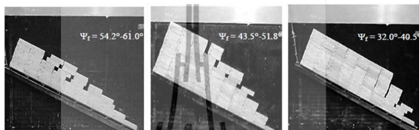
Figure 5. Some test results for various slope heights for S_H:S_V=1:4 .
