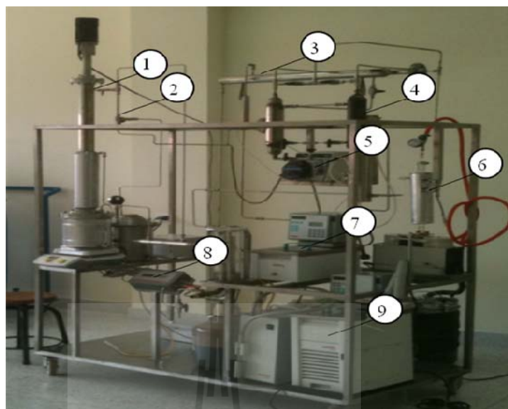
Figure 3.1 Setting apparatus of forced-mixing distillation, vapor permeation and pressure swing adsorption: 1, distillation column; 2, condenser; 3, vapor permeation; 4, pressure swing adsorption; 5, feed pump; 6, condenser; 7, oil bath; 8, density meter; 9, refrigerated circulator.
