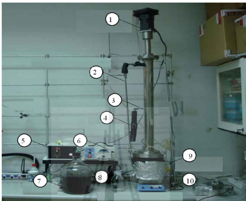
Figure 2.6 A high efficiency continuous distillation using forced-mixing column (Boontawan A., 2553): 1, motor; 2, condenser; 3, inlet; 4, heat exchanger; 5, speed controller; 6, feed pump; 7, feed solution; 8, product; 9, boiler; 10, ethanol heater.
