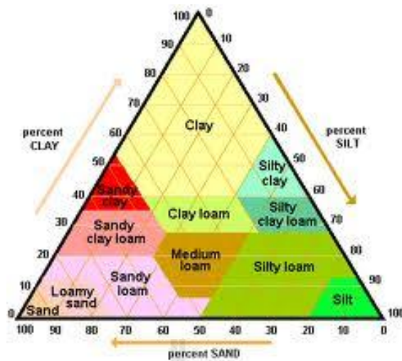
Figure 2.1 Textural triangle showing a soil's textural class according to the percentage of sand, silt and clay it contains.
