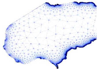
Fig.1 Unstructured mesh for complex geometry.
