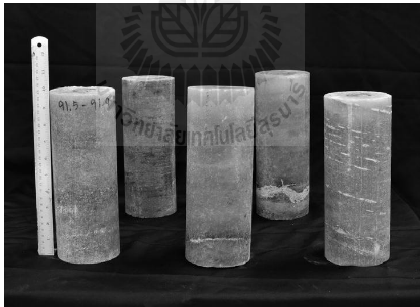
Figure 3.2 Some cylindrical salt specimens prepared for the uniaxial creep test.
