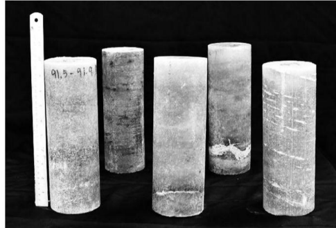
Figure 1. Some cylindrical salt specimens prepared for the uniaxial creep testing.
