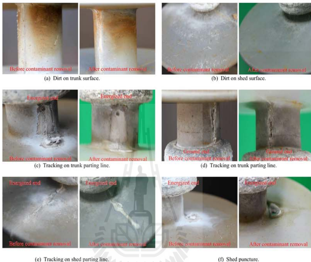
Fig. 5 Surface damage of tested specimens.
