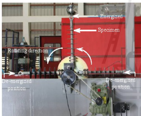
Fig. 3 Specimen arrangement during salt water dip wheel test
