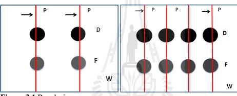
**Figure 3.1** Pen design (F: Feeding area; D: Drinking area; P: Perching area; W: Wall area). Fig.(left side): group size of 50 birds, Fig.(right size): group size of 100 birds
