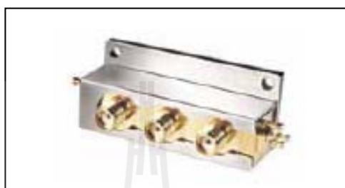
Figure 5.16 Photograph of RF-switch.
