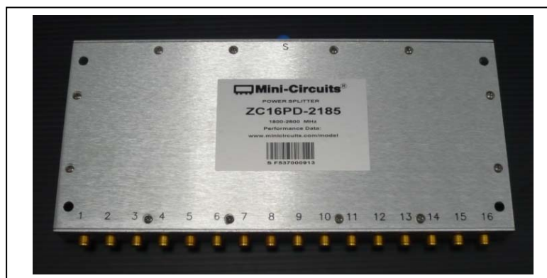
Figure 5.25 Photograph of 16:1 power combiner.
