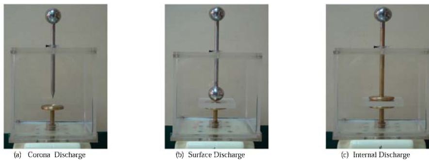
Fig. 6. Electrode Configuration for Partial Discharge Generation Source.
