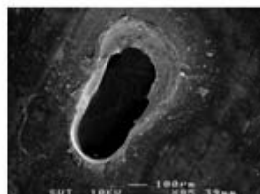
Fig. 11. Surface Damaged due to Electric stress 140kV/mm (1 s) at 23°C
