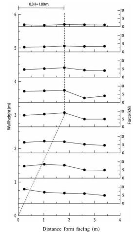
Figure 7. Measured tensions in the bearing reinforcement at 14 days after the end of construction
