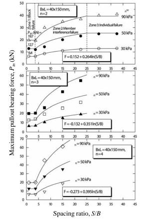
Figure 4. Effect of spacing ratio on pullout bearing resistance of the bearing reinforcement (Horpibulsuk and Niramitkornburee, 2010)
