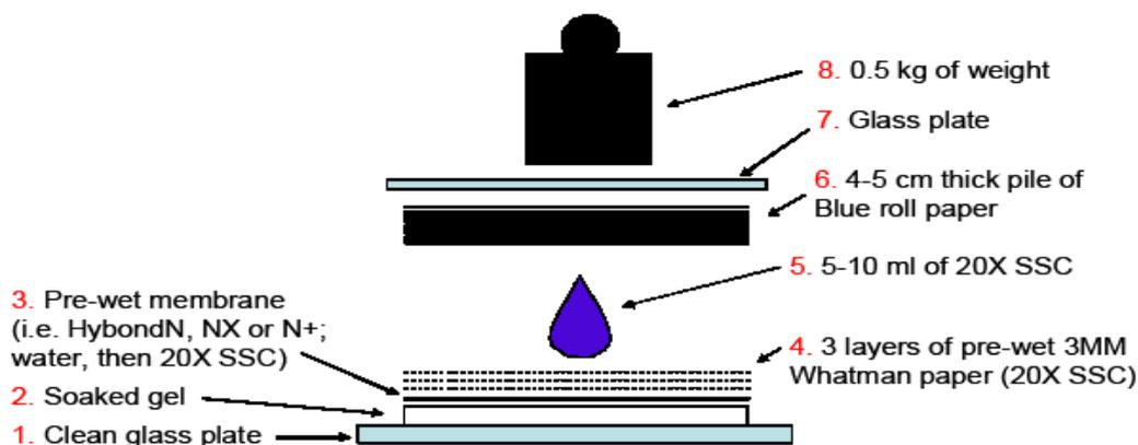
**Figure 13** Capillary blotting without reservoir followed the protocol of Molnár et al. (2007). The system was setup following the numbers and the transfer of RNA was done overnight.
