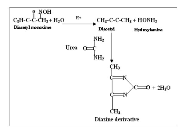
Figure 3.2 The principle of plasma urea nitrogen (PUN) determination
