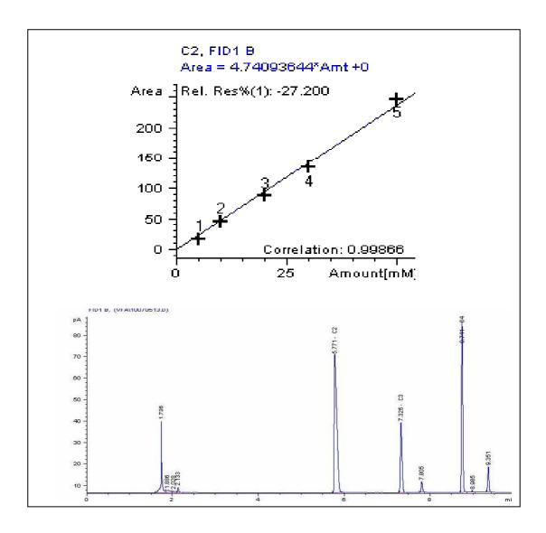
Figure 3.4 The relationship between C2 concentration and area in the C2 standard solution and the order of C2, C3, C4 arising.
