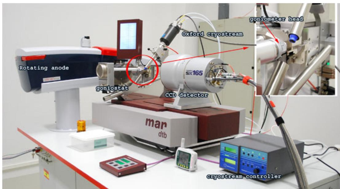
**Figure 2E** PX diffractometer consisting of rotating anode, CCD detector, Oxford cryostream, and the goniostat on the Macromolecule Crystallography end station at the Synchrotron Light Research Institute (Public Organization) (SLRI), Thailand.
