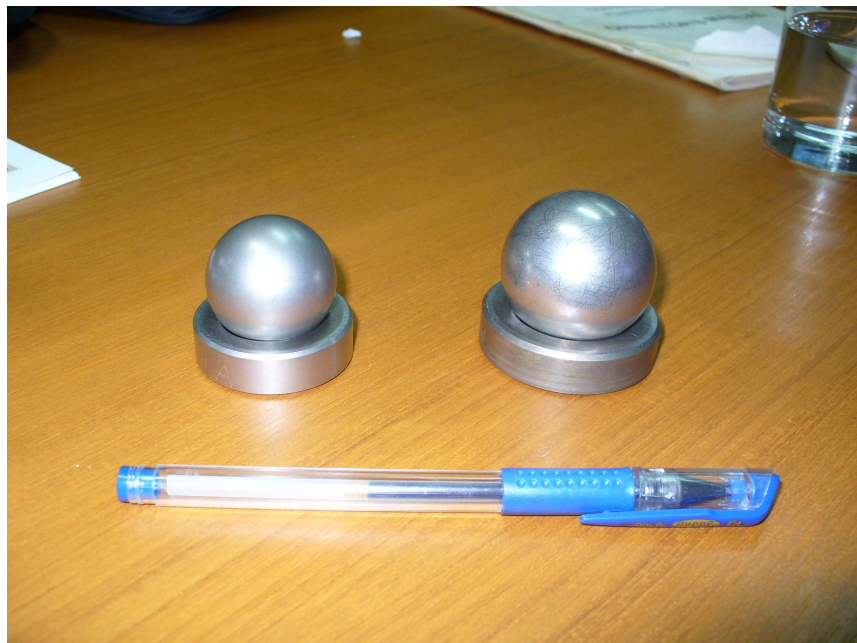
Figure 2.30 Lufkin's ball valves of sucker rod pump in U Thong oil fields.
