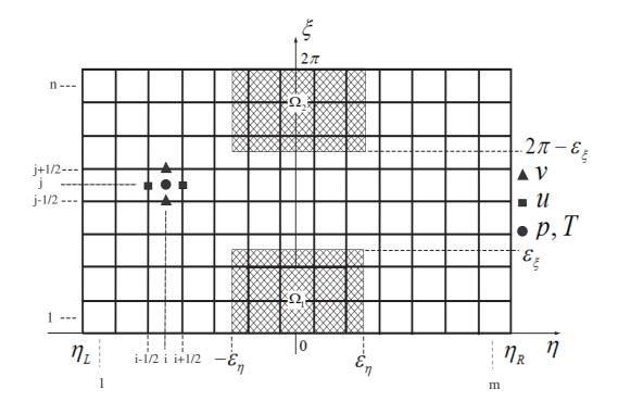
Figure 3.2 Staggered arrangement of v, u, p and T.
