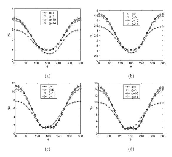
Figure 5.1 Local Nusselt number for different gap spacing at Re = 20,  $\alpha = 0$ , and (a) Pr = 0.7, (b) Pr = 1, (c) Pr = 10, and (d) Pr = 20.
