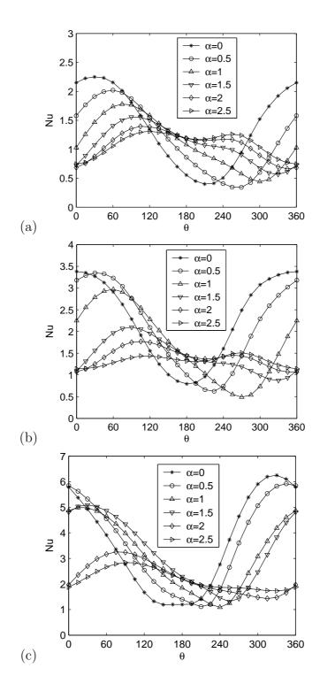
Figure 5.11 Local Nusselt number variation on the surface of the circular cylinders at Pr = 1, g = 1,  $\alpha = 0$ , 0.5, 1, 1.5, 2, and 2.5 for (a) Re = 10, (b) Re = 20, and (c) Re = 40.
