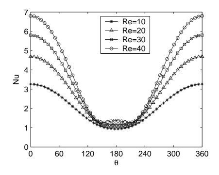
Figure 4.7 Local Nusselt number variation on the surface of the circular cylinders at Pr = 1, g = 14 at various Reynolds numbers.
