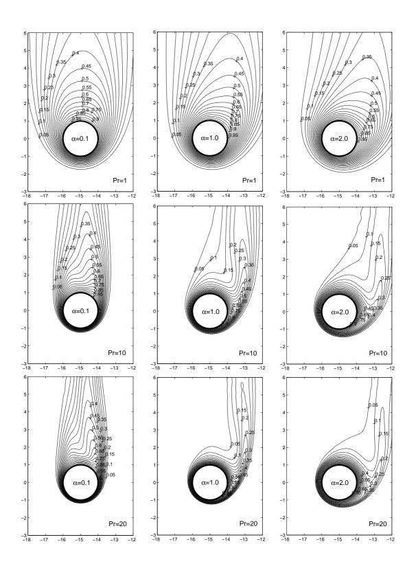
Figure 5.5 Temperature contours over two circular cylinders at Re = 20, g = 14,  $\alpha = 0.1$ , 1.0, 2.0, and for Pr = 1, 10, and 20.
