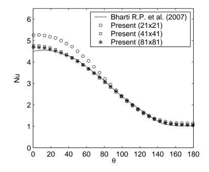
Figure 4.8 Local Nusselt number on the sequence of grids for Re = 20, g = 14, and Pr = 1.
