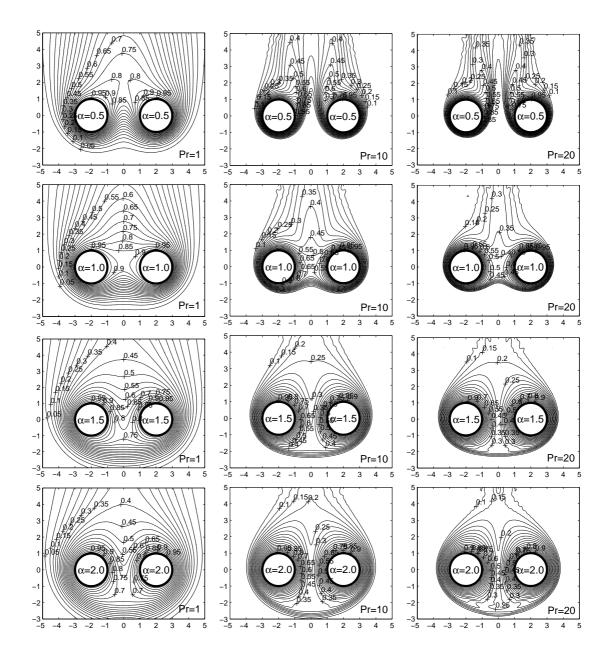
Figure 5.14 Temperature contours over two circular cylinders at Re = 20, g = 1, Pr = 1, 10, 20, and  $\alpha = 0.5$ , 1.0, 1.5, and 2.0.
