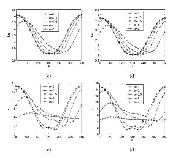
Figure 5.3 Local Nusselt number variation on the surface of the circular cylinders at Re = 20, g = 14,  $\alpha = 0$ , 0.1, 0.5, 1, and 2 for (a) Pr = 0.7, (b) Pr = 1, (c) Pr = 10, and (d) Pr = 20.
