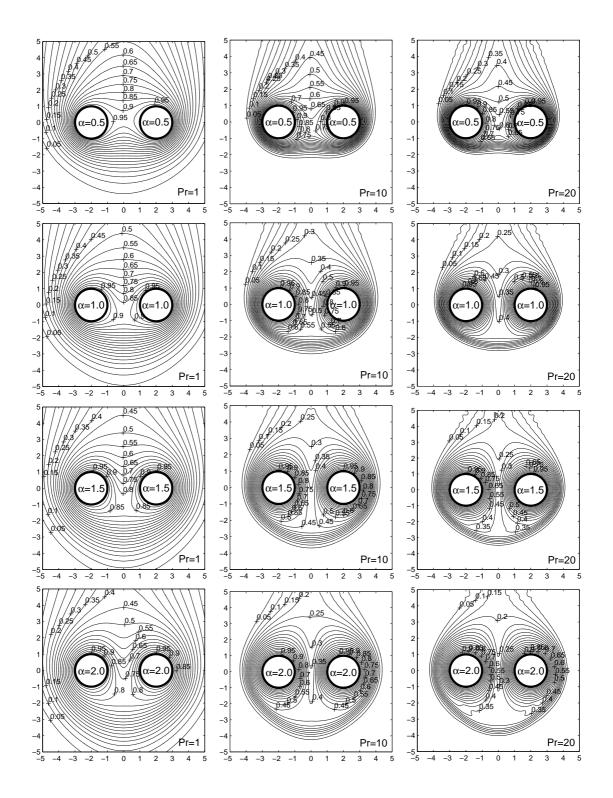
Figure 5.13 Temperature contours over two circular cylinders at Re = 10, g = 1, Pr = 1, 10, 20, and  $\alpha = 0.5$ , 1.0, 1.5, and 2.0.
