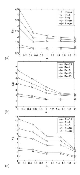
Figure 5.15 Nusselt number at (a) Re = 10, (b) Re = 20, and (c) Re = 40, and g = 1 for different Prandtl number Pr.
