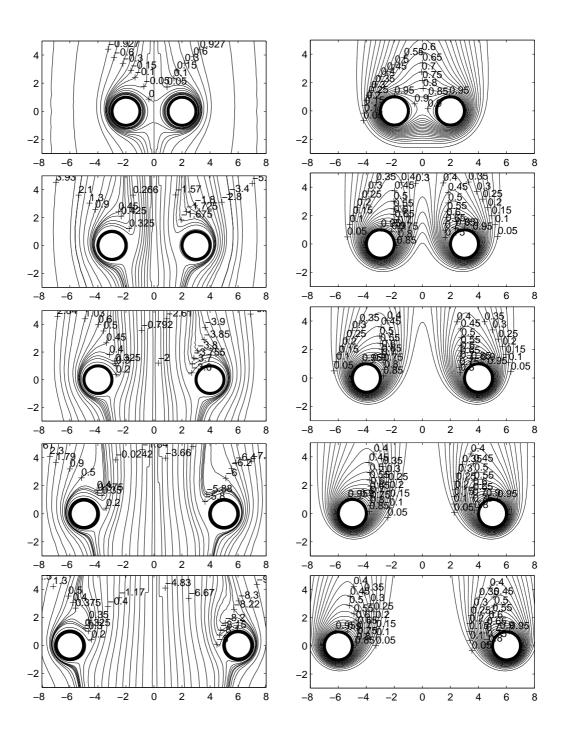
Figure 5.8 Streamline patterns (left column) and temperature contours (right column) of flow over two circular cylinders at Re = 20,  $\alpha = 1$ , and g = 1 - first row, g = 2 - second row, g = 3 - third row, g = 4 - fourth row, and g = 5 - fifth row.
