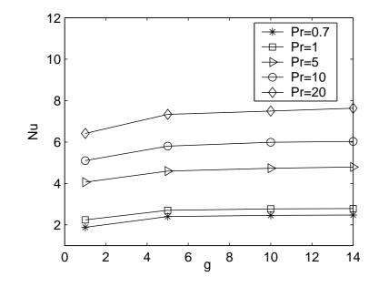
Figure 5.2 Average Nusselt number for different gap spacing at Re = 20,  $\alpha = 0$ .
