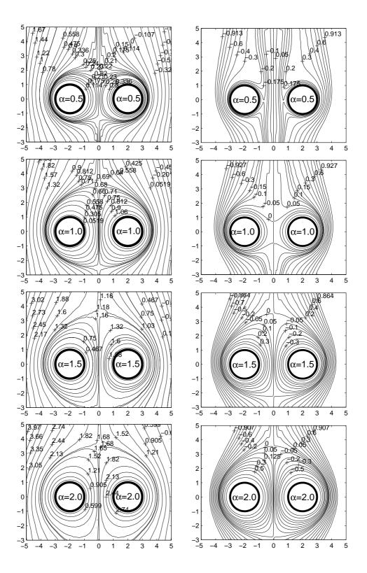
Figure 5.12 Streamlines contours over two circular cylinders at Re = 10 (left column), and Re = 20 (right column), Pr = 1, g = 1, and  $\alpha = 0.5$ , 1.0, 1.5, and 2.0.
