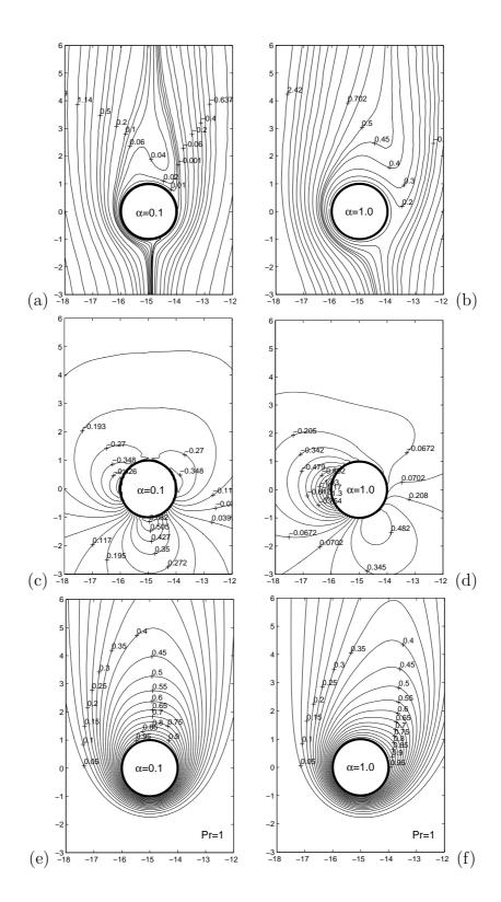
Figure 4.9 (a-b) Streamline patterns, (c-d) pressure fields and (e-f) temperature contours of flow over two circular cylinders at Re = 20, g = 14, and Pr = 1.0, left column:  $\alpha = 0.1$ , right column:  $\alpha = 1.0$ .
