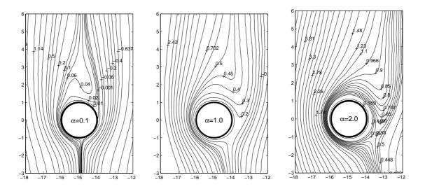
Figure 5.4 Streamline patterns at Re = 20, g = 14,  $\alpha = 0.1$ , 1.0, and 2.0, and for Pr = 1.
