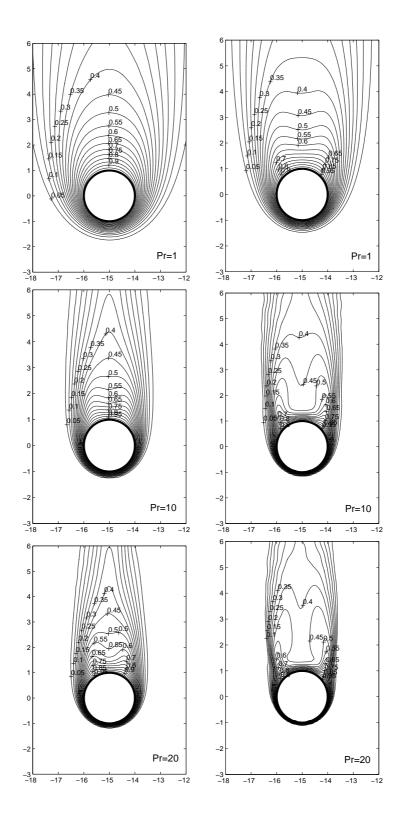
Figure 4.3 The temperature contours for  $1^{st}$ -column: Re = 20 and  $2^{nd}$ -column: Re = 40 of flow over two circular cylinders for g = 14,  $\alpha = 0$  at  $1^{st}$ -row: Pr = 1,  $2^{nd}$ -row: Pr = 10, and  $3^{rd}$ -row: Pr = 20.
