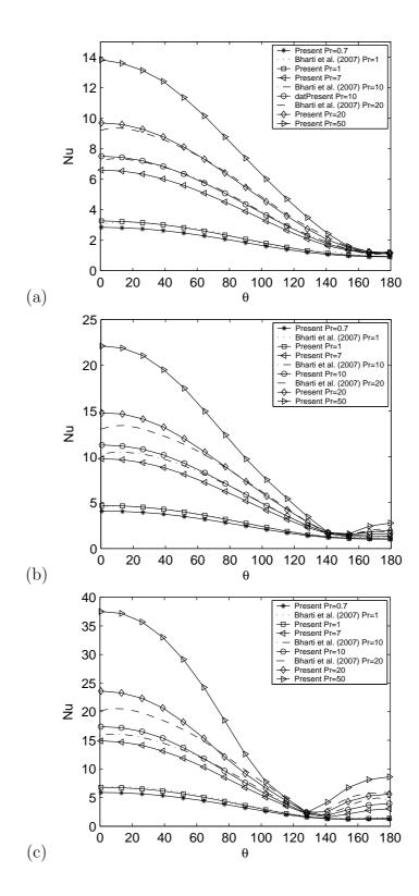
Figure 4.6 Local Nusselt number variation on the surface of the circular cylinders for  $\alpha = 0$ , g = 14, and (a) Re = 10, (b) Re = 20, (c) Re = 40 at various Prandtl numbers.
