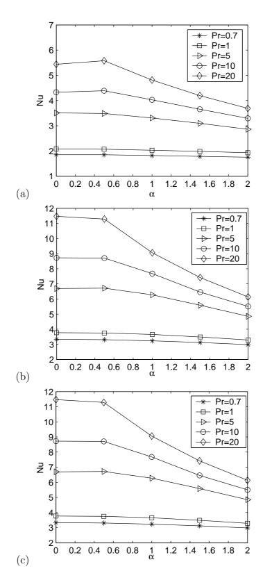
Figure 5.6 Nusselt number at (a) Re = 10, (b) Re = 20, and (c) Re = 40, and g = 14 for different Prandtl number Pr.
