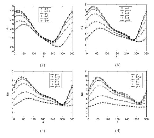
Figure 5.7 Local Nusselt number at Re = 20,  $\alpha = 1$ , and (a) Pr = 1, (b) Pr = 5, (c) Pr = 10, and (d) Pr = 20.
