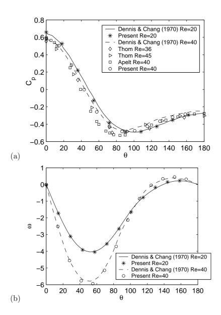
Figure 4.1 (a) Pressure coefficient over cylinder surface, (b) the vorticity distribution over cylinder surface, for the left cylinder at Re = 20, 40, and g = 14.
