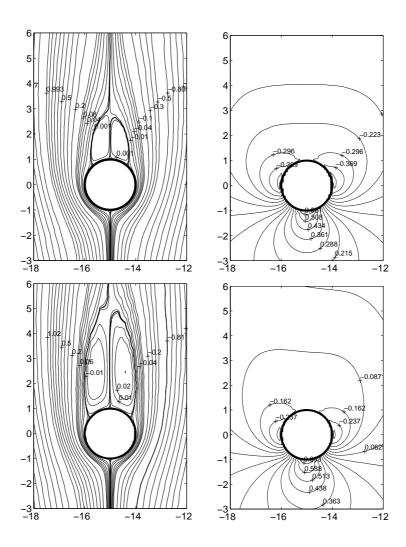
**Figure 4.2** 1<sup>st</sup>-column: Streamline patterns, 2<sup>nd</sup>-column: pressure fields of flow over two circular cylinders for g = 14,  $\alpha = 0$  at 1<sup>st</sup>-row: Re = 20, 2<sup>nd</sup>-row: Re = 40.
