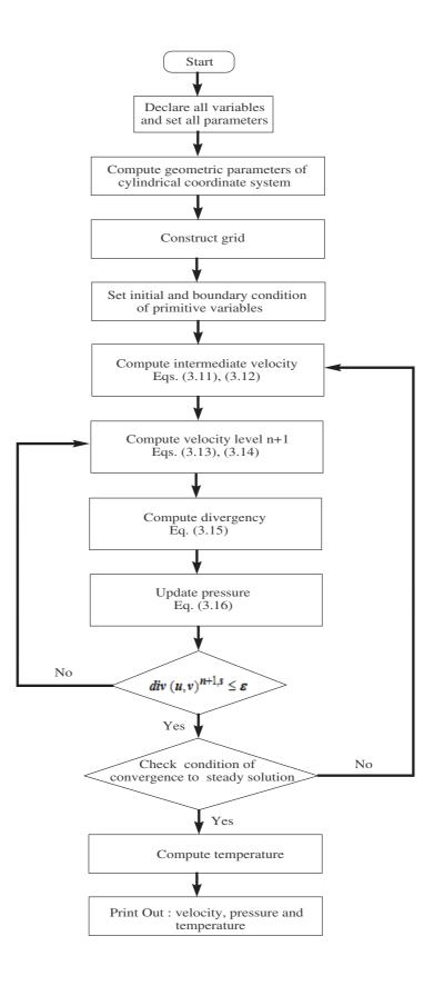
Figure 3.4 The flow chart of the numerical algorithm.
