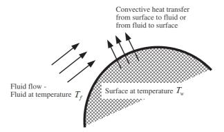
Figure 2.2 Convective heat transfer from a surface.
