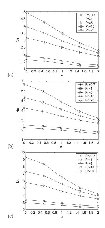
Figure 5.10 Nusselt number at (a) Re = 10, (b) Re = 20, and (c) Re = 40, and g = 2 for different Prandtl number Pr.
