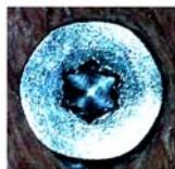
Figure 3. Example photo of head slot of damage screw
