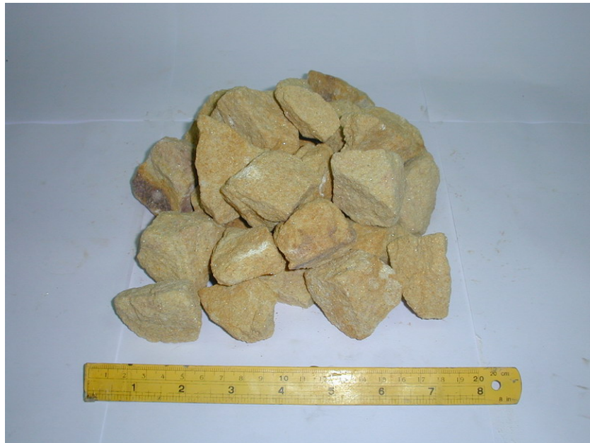
Figure 4.8 Example of rock fragments of Phra Wihan sandstone prepared for slake durability index test.
