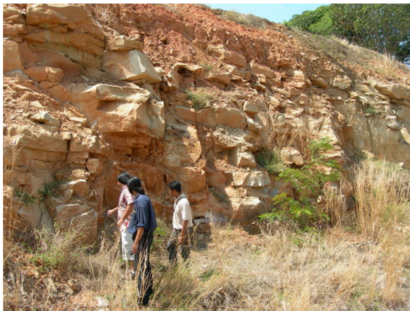
Figure 3.3 White quartz sandstone collected from the embankment of Thep Sathit-Chaiyaphum highway at km 287. The slope was excavated in 2003.
