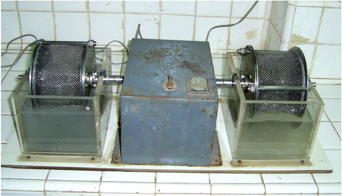
Figure 4.1 Slake durability test apparatus.
