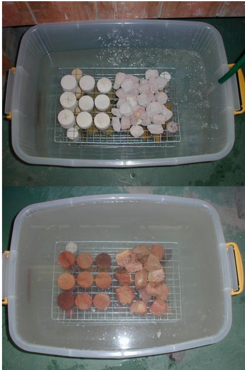
Figure 4.10 Specimens of rock disks and fragments submerged under water tank at 25°C.
