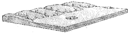
(A) An offshore island acts as a breakwater to incoming waves and creates a wave shadow along the coast behind it.
