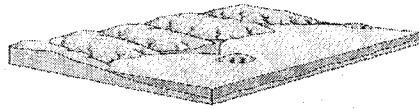
(B) Sediment moved by longshore drift is trapped in the shadow zone.
