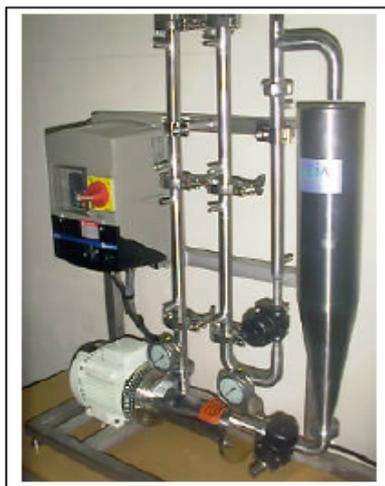
Figure 3.1 Microfiltration unit.
