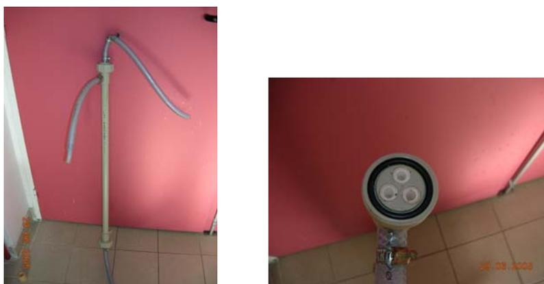
Figure 3.2 Tubular module and membranes.
