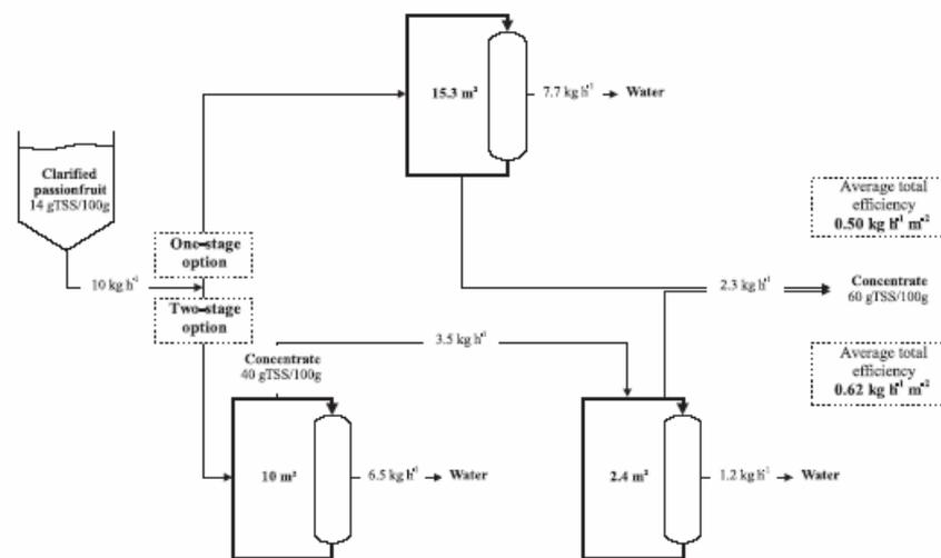
Figure 2.7 Scheme of one- or two-stage continuous-feed OE process and membrane area required (Vaillant et al., 2001).
