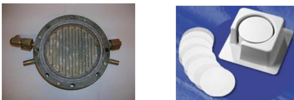
Figure 3.3 Flat module and membranes.
