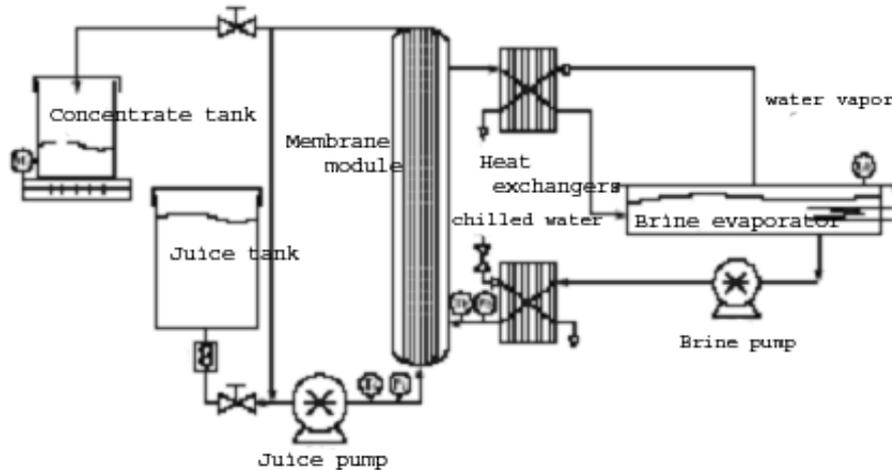
**Figure 2.6** Scheme of the industrial pilot plant of OE (Vaillant et al., 2001).
