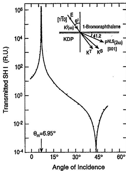
FIG. 6. The total transmitted second harmonic intensity  $I_{\text{total}}(2w) = I_S(2w) + I_T(2w)$  as a function of angle of incidence  $\theta_i$ . The phase matching angle  $\theta_i^m = 6.95^\circ$  and the dip of  $I_{\text{total}}(2w)$  at  $44.0^\circ$ .
