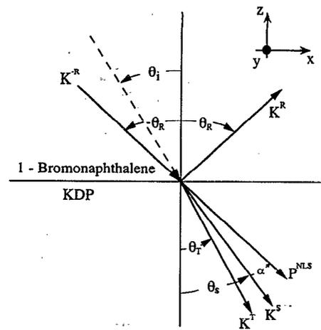
FIG. 5. Null transmitted inhomogeneous second harmonic generation where  $\alpha + \theta_S + \theta_R = 0$ . The  $\mathbf{P}^{NLS}(2\omega)$  source cannot radiate in the medium in the direction  $\mathbf{K}^{-R}$  which would otherwise yield transmitted inhomogeneous second harmonic wave.
