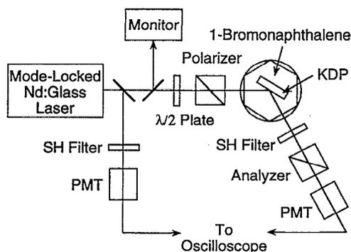
FIG. 2. Experimental arrangement for measuring transmitted SHG.
