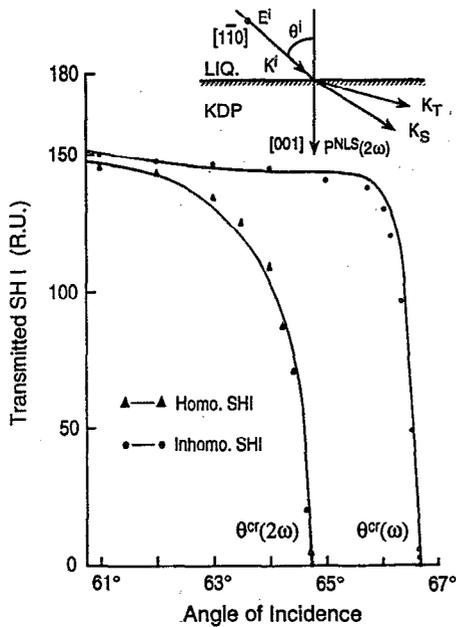
FIG. 3. The intensities of inhomogeneous and homogeneous transmitted second harmonic waves in the neighborhood of critical angle  $\theta^{cr}(w)$  and  $\theta^{cr}(2w)$ .
