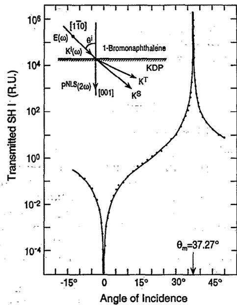
FIG. 4. The total transmitted second harmonic intensity  $I_{\text{total}}(2w) = I_S(2w) + I_T(2w)$  as a function of angle of incidence  $\theta_i$ .  $I_S(2w) = I_T(2w) = 0$  at  $\theta_i = 0$  and phase matching angle  $\theta_m^* = 37.27^\circ$ .
