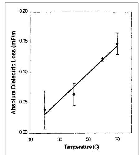
**Fig. 6**—Representative data and straight line regression giving dielectric loss of stabilized mince as a function of temperature. 77% moisture; 0.74% salt concentration.
