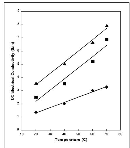
Fig. 3b—Representative data and straight line regression, showing DC electrical conductivity of surimi paste as a function of temperature and salt. 79% moisture content; salt concentration: 1% (◆); 2% (■); 3% (▲).
