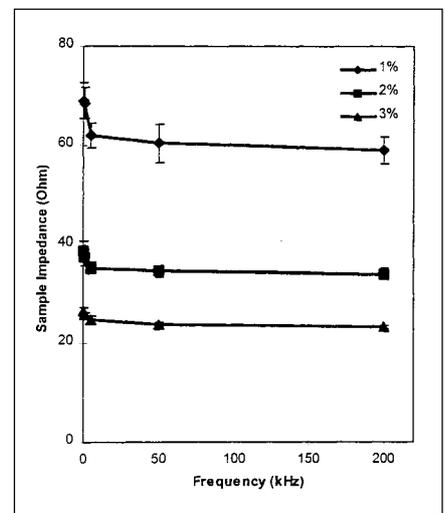
Fig. 3a—Representative data giving sample impedance of surimi paste as a function of frequency and salt. 79% moisture content; 40°C; salt concentration: 1% (◆); 2% (■); 3% (▲).
