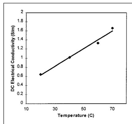
**Fig. 5**—Representative data and straight line regression giving DC conductivity of stabilized mince as a function of temperature. 77% moisture content; 0.74% salt concentration.
