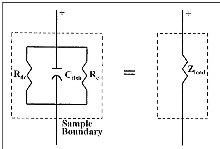
Fig. 1—Equivalent circuit representing food sample.
