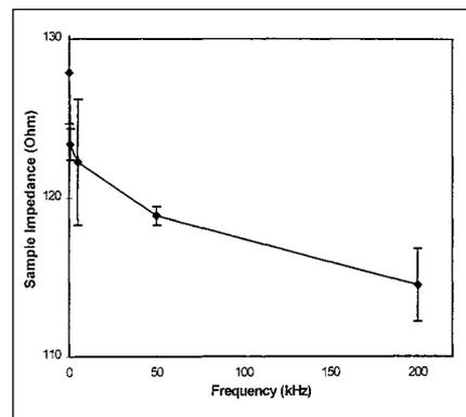
**Fig. 4**—Representative data giving sample impedance of stabilized mince as a function of frequency. 77% moisture content; 0.74% salt concentration; 40 $^{\circ}$ C.
