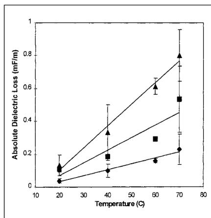
**Fig. 3c**—Representative data and straight line regression showing dielectric loss factor of surimi paste as a function of temperature and salt. 79% moisture content; salt concentration: 1%( $\blacklozenge$ ); 2%( $\blacksquare$ ); 3%( $\blacktriangle$ ).
