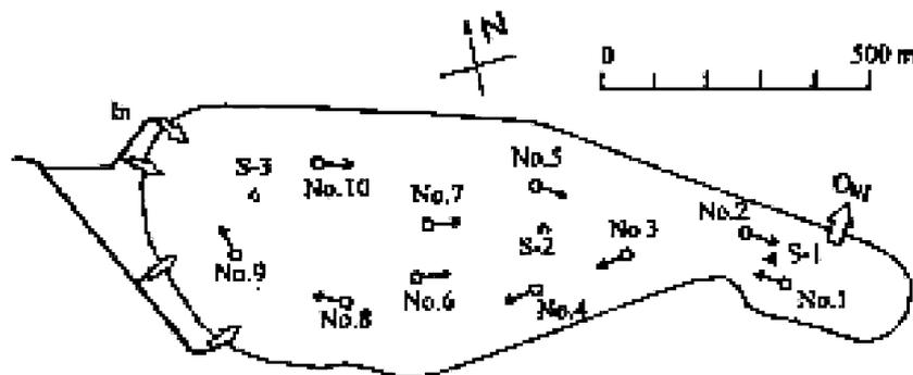
Figure 1. Sampling sites and the location of the ten USRS units arranged in Lake Senba, symbols: O; USRS,  $\Delta$ ; sampling sites. Arrows show the direction of the water jet current generated by USRS (Nakano *et al.* 2001).
