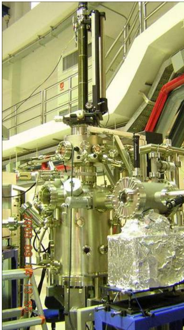
Fig. 3.1 Photoemission system shown above is an experimental station of the BL4 beamline.
