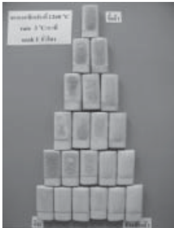
Figure 3. Glaze fired under condition #1; maximum temperature 1,260°C; heating rate 3°C/min; soaking time 1 h under oxidation
