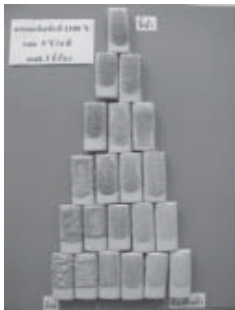
Figure 5. Glaze fired under condition #3; maximum temperature 1,300°C; heating rate 5°C/min; soaking time 3 h under oxidation
