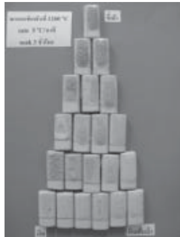
Figure 4. Glaze fired under condition #2; maximum temperature 1,260°C; heating rate 5°C/min; soaking time 3 h under oxidation
