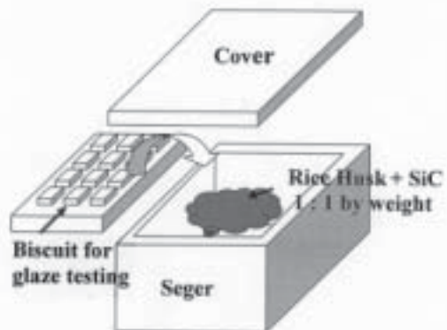
Figure 2. Crucible setting for reducing firing condition
