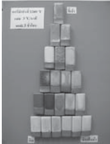
Figure 7. Glaze fired under condition #5; maximum temperature 1,260°C; heating rate 3°C/min; soaking time 3 h under reduction
