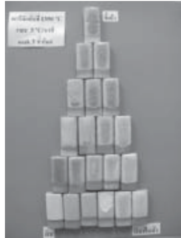
Figure 8. Glaze fired under condition #6; maximum temperature 1,350°C; heating rate 5°C/min; soaking time 3 h under reduction
