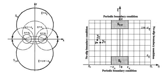
Figure 2. Transformation between physical domain and computational domain
