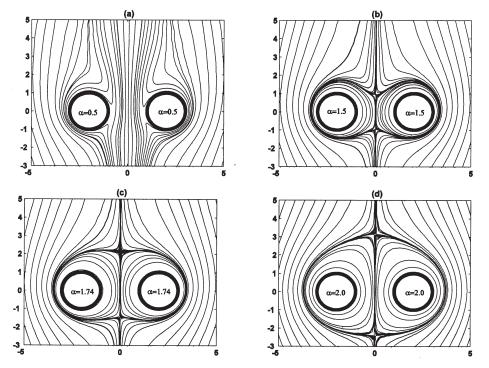
Figure 7. Streamline patterns of flow over two circular cylinders at Re = 20, g = 1 and  $\alpha = 0.5$ , 1.5, 1.74, 2.0
