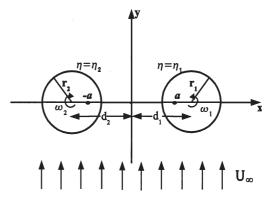
Figure 1. Geometrical sketch of the flow scheme
