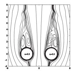
Figure 4. Streamline patterns of flow over two circular cylinders at Re = 40, g = 1and  $\alpha = 0.0$
