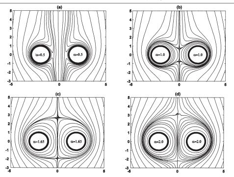
Figure 6. Streamline patterns of flow over two circular cylinders at Re = 10, g = 1 and  $\alpha = 0.5$ , 1.0, 1.65, 2.0
