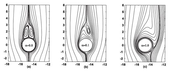
Figure 3. Streamline patterns of flow over two circular cylinders at Re = 20, g = 14 and  $\alpha = 0.0, 0.1, 1.0$
