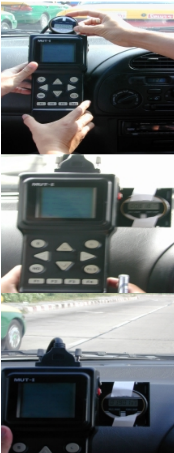
Figure C.2 Mut-II measuring driving parameters
