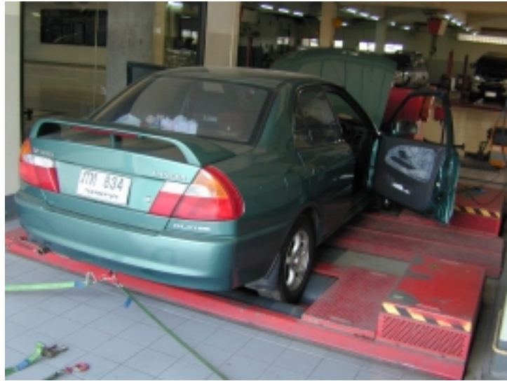
Figure C.9 View of test car on fixed on chassis dynamometer
