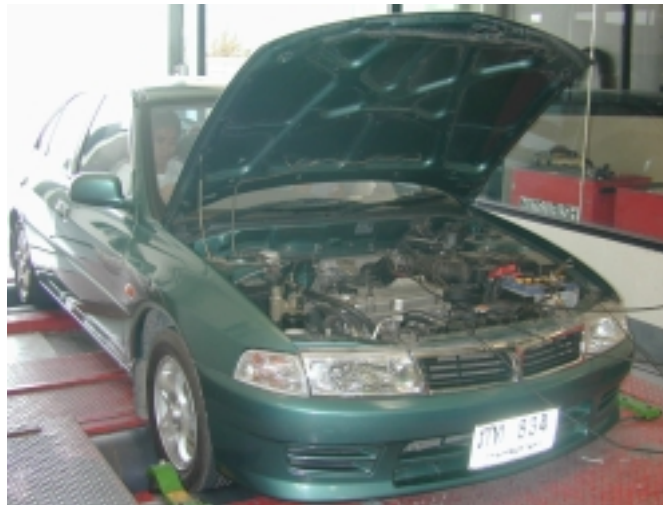
Figure 3.6 Driving simulation on chassis dynamometer with pollutants measuring
