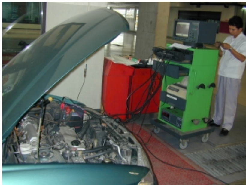
Figure C.7 Test cars was set on chassis dynamometer
