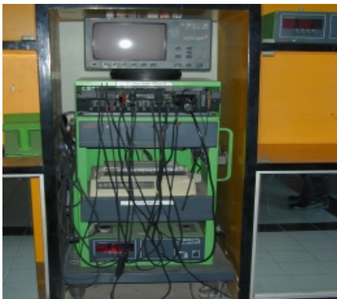
Figure 3.4 Exhaust Gas Analyzer for CO, HC, CO 2
