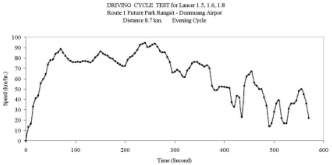
Figure 4.7 Driving cycle for Lancer 1.5, 1.6, and 1.8 on Route 1 Future Park Rangsit-Donmuang (Distance 8.7 km.) Evening Cycle
