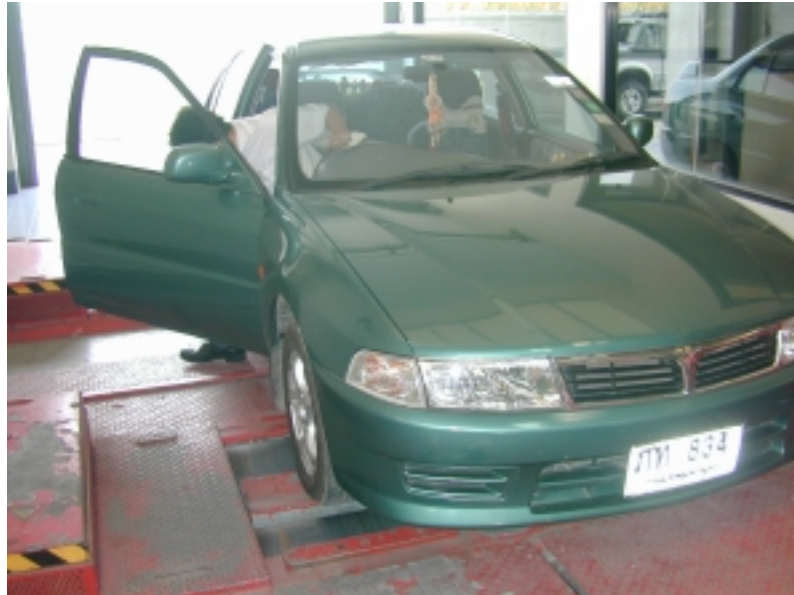
Figure C.7 Test cars was set on chassis dynamometer
