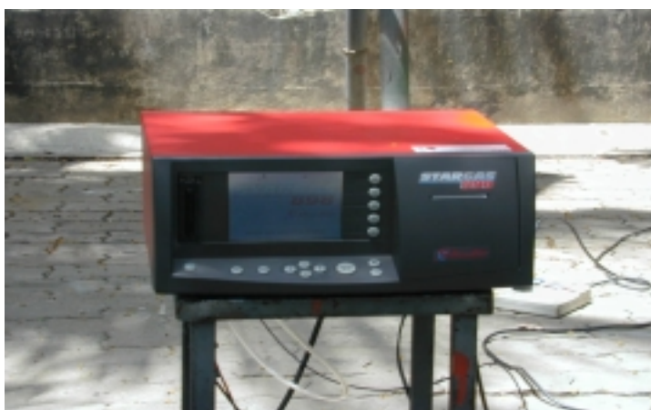
Figure 3.4 Exhaust Gas Analyzer for CO, HC, CO 2
