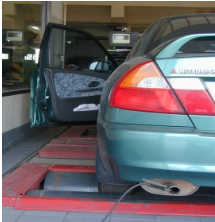
Figure C.9 View of test car on fixed on chassis dynamometer
