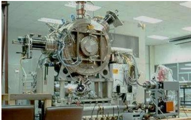
Fig.3.4 The RF cavity in STR
