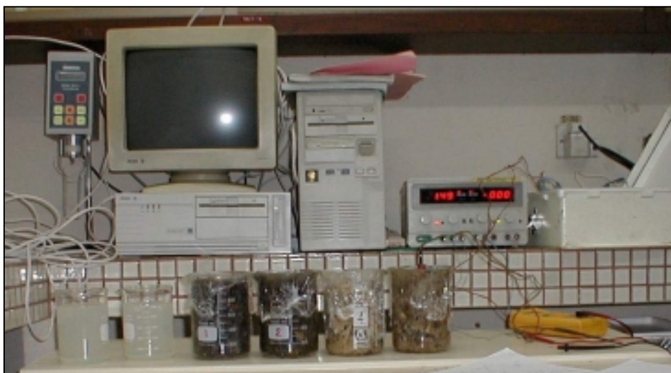
Figure 3.16 Thermal conductivity measurement at AIT
