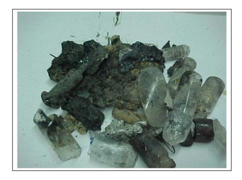
**Figure 4.2.** Bottom ash components with particles size range of > 9.5 mm
