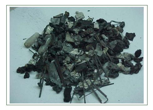
Figure 4.3. Bottom ash components with particle size of 4.75-9.5 mm
