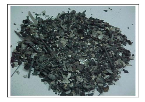
Figure 4.4. Bottom ash components with particle size of 0.5-4.75 mm
