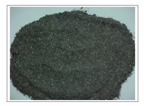
Figure 4.5. Bottom ash components with particle size of <0.5 mm
