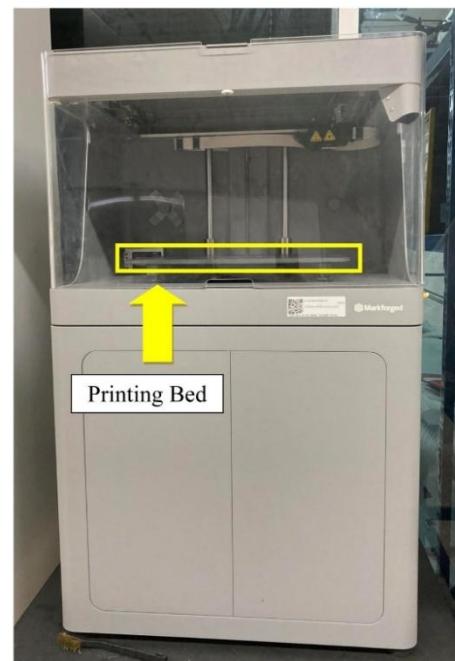
Fig. 1. Markforged X7 3D printer printing specimens.
