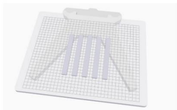
Fig. 2. Visualization of laying specimen on Markforged X7 printing bed.
