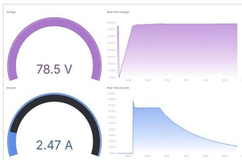
Figure 9. Real-time CC–CV charging profile of the 72 V, 15 A NMC configuration visualized using Grafana. The upper plots show the voltage evolution, while the lower plots show the current behavior. The transition from constant-current (CC) to constant-voltage (CV) operation is clearly observable.
