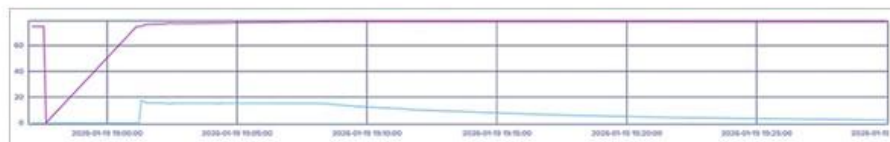
Figure 8. Real-time voltage and current data of the 72 V 15 A charging profile visualized directly using the native InfluxDB query interface. The purple curve represents the battery terminal voltage, while the blue curve denotes the charging current. Although the data are accurately recorded, the visualization is mainly intended for data inspection rather than operator-oriented monitoring.
