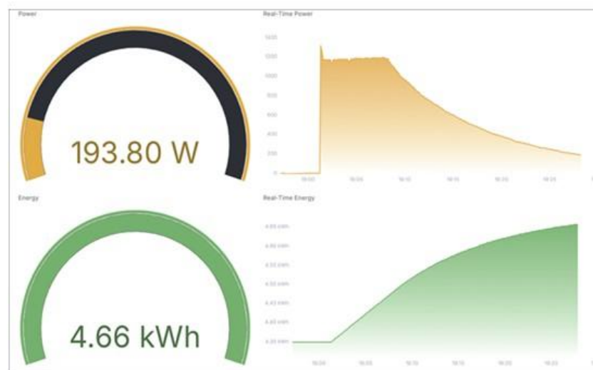
Figure 10. Power & Energy Dashboard (Grafana, 72 V 15 A).
