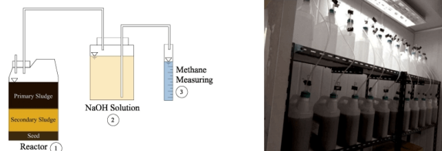
Figure 3 Installation of the BMP Test consists of 1) reaction tank, 2) container containing NaOH solution, and 3) graduated container for measuring the volume of NaOH solution replaced by methane gas.
