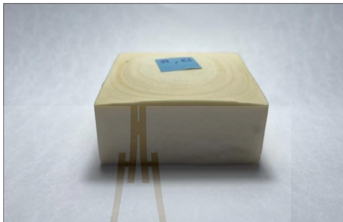
Figure 3.2 Sample cube specimen of 50 mm X 50 mm X 25 mm used in the study.
