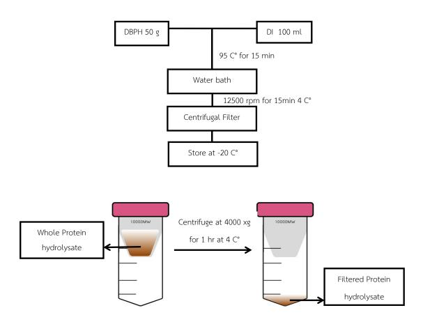
Figure 3.1 Filtration of Duck Blood Protein Hydrolysate.
