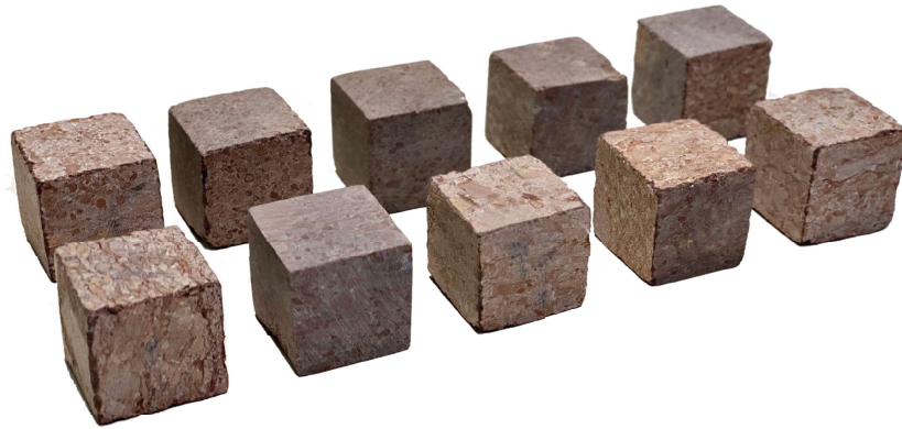
Figure 3.3 Examples of PPCS specimens prepared for dry testing.
