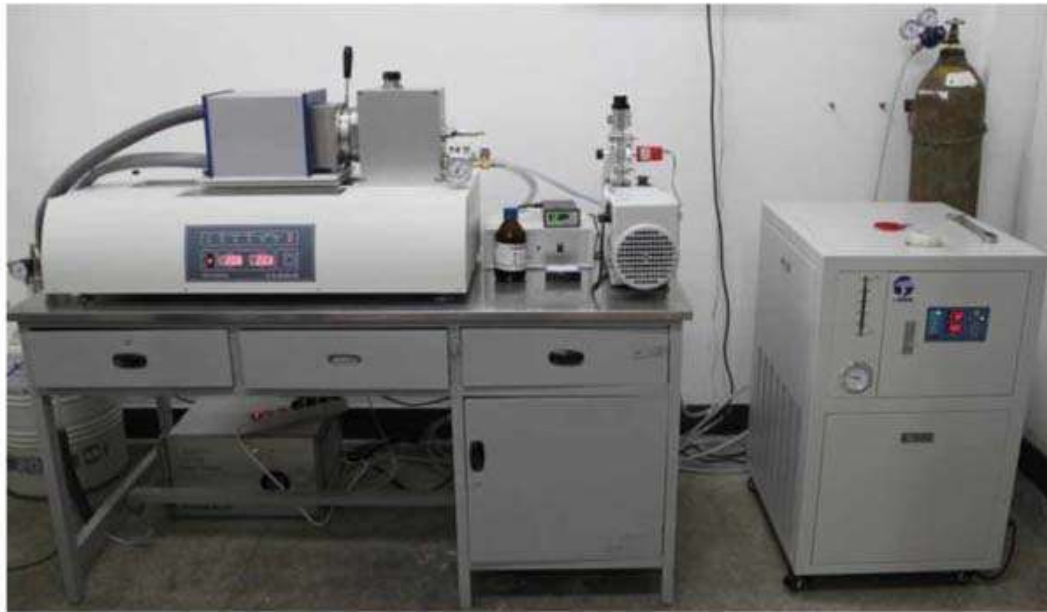
Figure 47 LINSEIS LSR-3 Seebeck type resistivity measurement system.
