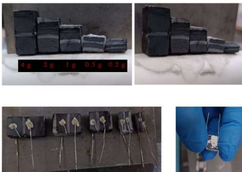
Figure 40 The test cells of monolithic \beta - \text{Zn}_4\text{Sb}_3/\text{ZnO} TEGs versus weight size of \beta - \text{Zn}_4\text{Sb}_3 pellets part.
