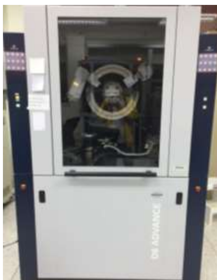
Figure 43 Shows X-ray diffraction machine, D8-Bruker, SUT.
