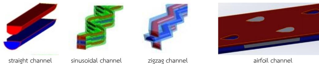
**Figure 2.5** Different kinds of PCHE flow channels (Kim et al., 2015; Saeed et al., 2020).
