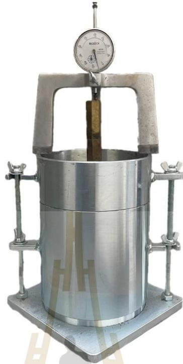
Figure 5.12 Swelling test setup in compaction mold.
