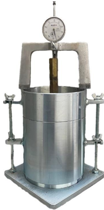
Figure 5.12 Swelling test setup in compaction mold.
