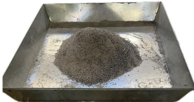
Figure 5.1 Fine-grained stone dust mixed with bentonite prepared in plastic tray.
