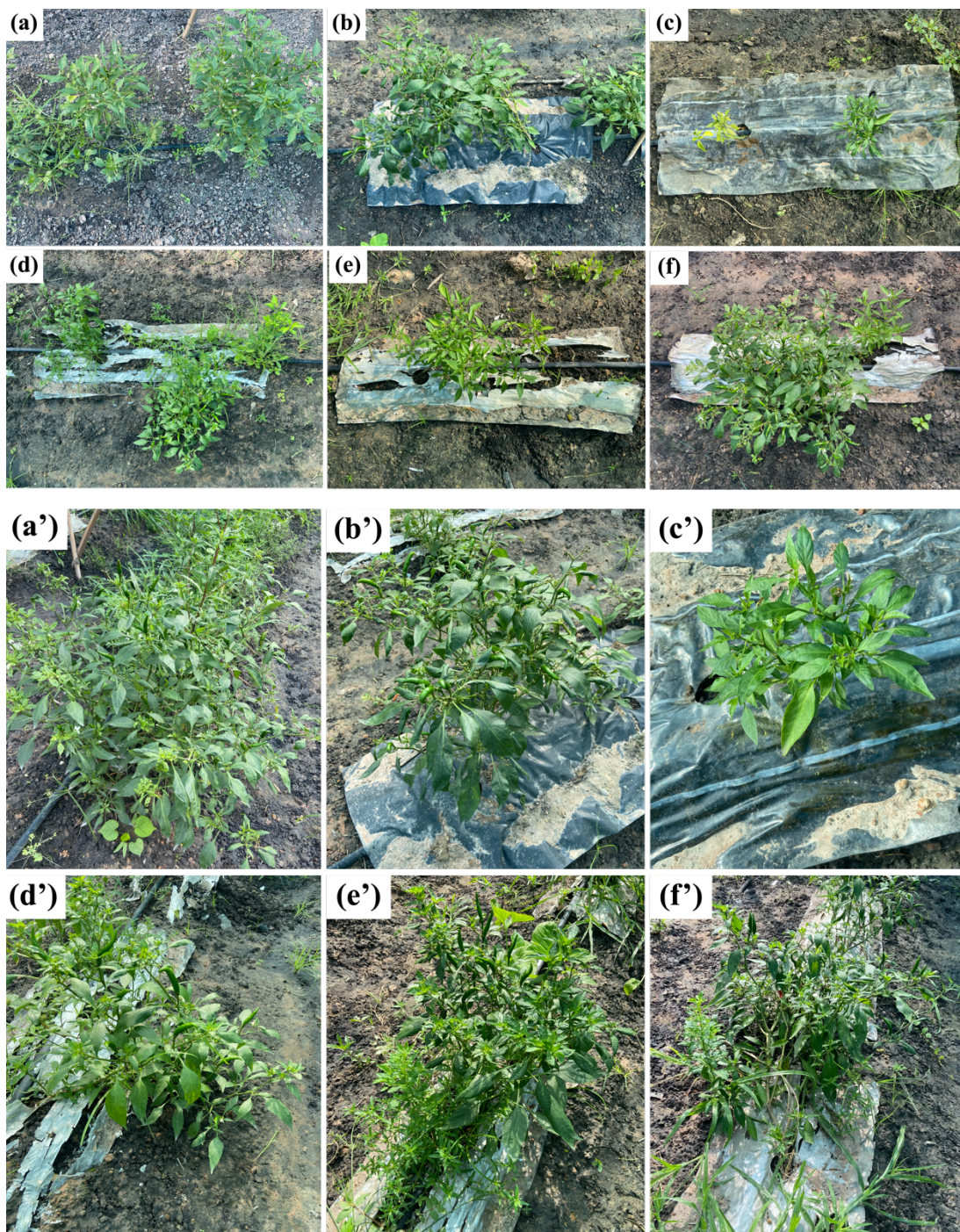
Figure 4.35 Chilli planting without mulch film (a, a') and with various types of mulch films: HDPE (b, b'), neat PLA (c, c'), PLA/NR blend (d, d'), PLA/NR/3%RS (e, e'), and PLA/NR/5%RS (f, f') biocomposite films at 3 months of cultivation.
