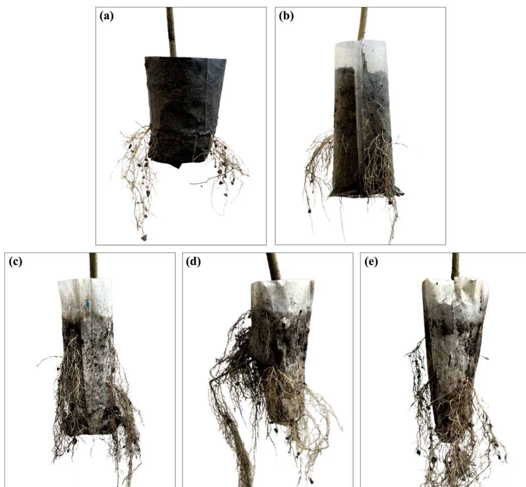
Figure 4.24 The growth of chili plant's root from seedling bags made from HDPE (a), neat PLA (b), PLA/NR blend (c), PLA/NR/3%RS (d), and PLA/NR/5%RS (e) biocomposite films after planting for 3 months.
