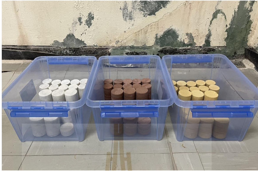
Figure 4.2 Specimens submerged in plastic containers.
