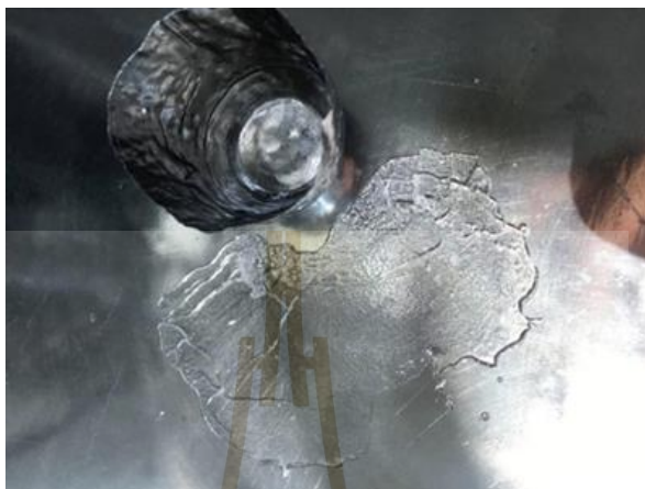
Figure 5.3 The prepared lithium borate glass by melt-quench technique.
