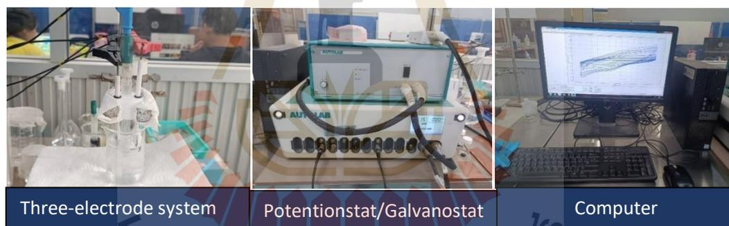
**Figure 3.9** Electrochemical measurement system includes a three-electrode system, potentionstat/galvanostat and a computer.
