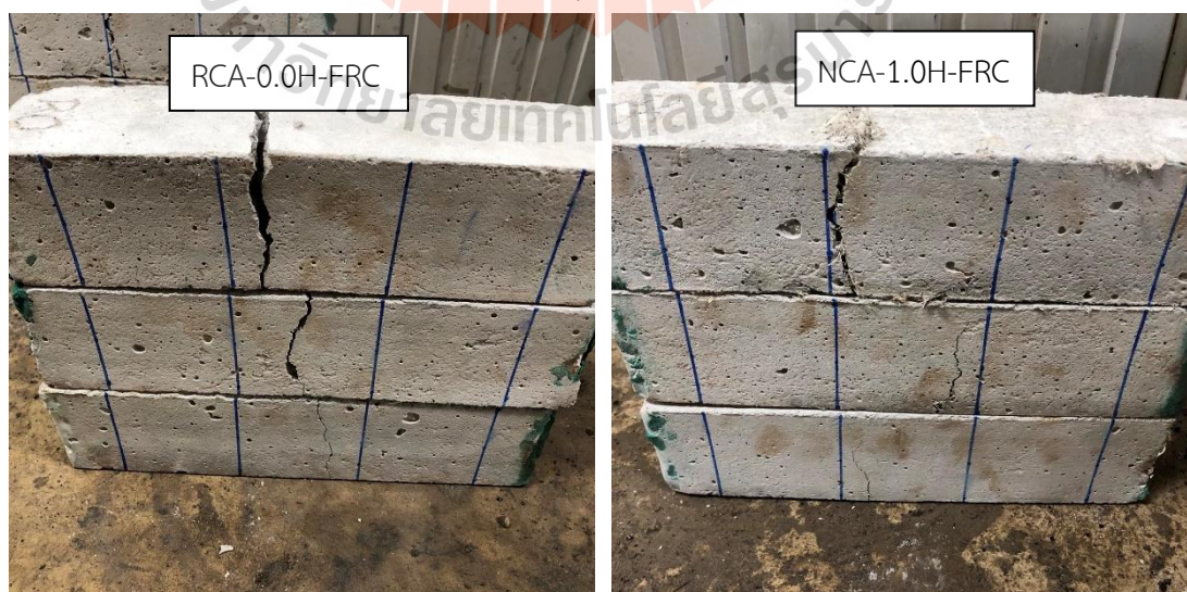
Figure 4.14 Flexural failure of hemp fiber reinforced concrete using NCA.
