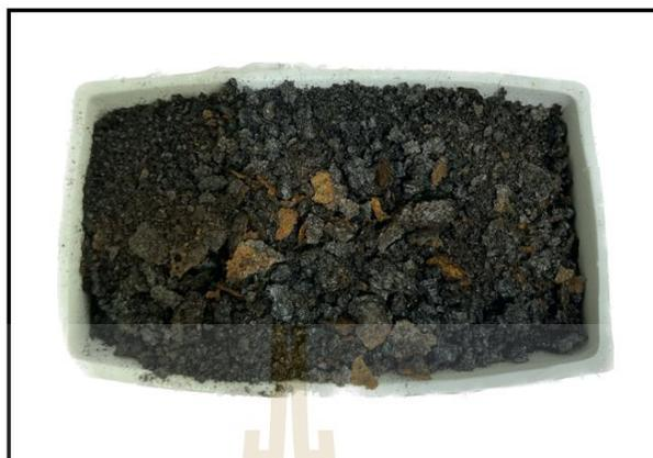
Figure 3.15 Black powder after calcination at 350°C
