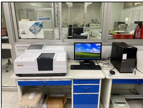
Figure 3.20 UV-Vis spectroscopy (UV-Vis, model: CARY 300)
