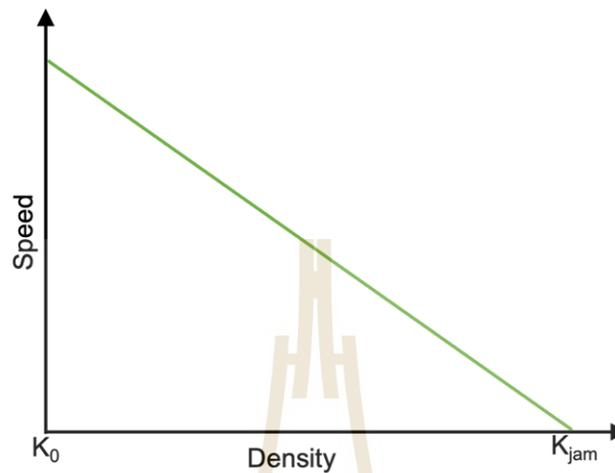
Figure 2.2 The Relationship Between Vehicle Speed and Traffic Density
