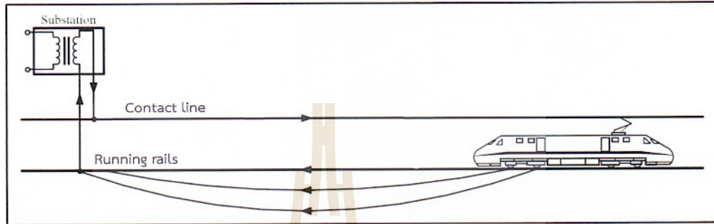
Figure 2.5 Direct feeding without return conductor.
