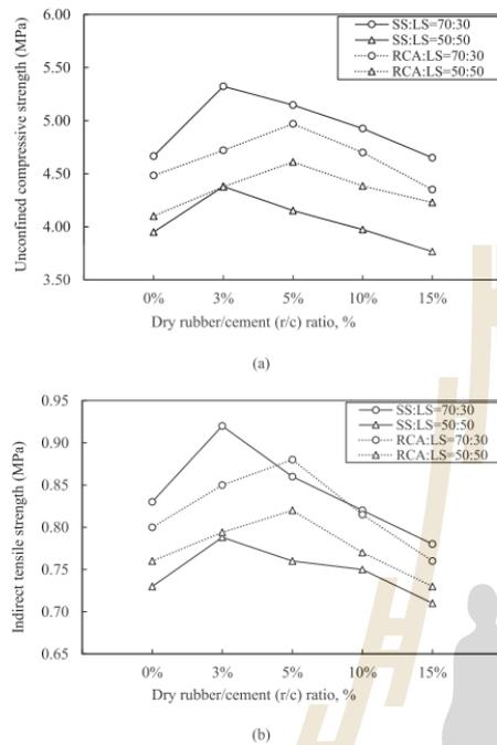
Fig. 3. (a) Unconfined compressive strength, and (b) Indirect tensile strength of 28-day cement- and cement-NRL stabilized SS:LS and RCA:LS samples at different SS/RCA:LS replacements and dry rubber/cement (r/c) ratios.
