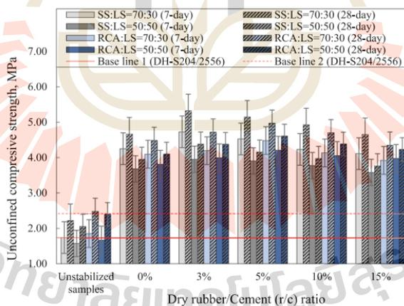
Fig. 3. Unconfined compressive strength of unstabilized samples, cement- and cement-NRL stabilized SS:LS and RCA:LS samples at various  $r/c$  ratios.
