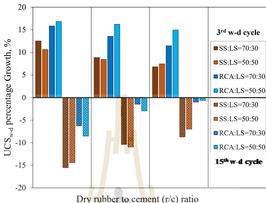
**Figure 5.5**  $UCS_{w-d}$  percentage growth of cement-NRL stabilized SS:LS and RCA:LS samples at the 3<sup>rd</sup> and 15<sup>th</sup> w-d cycles
