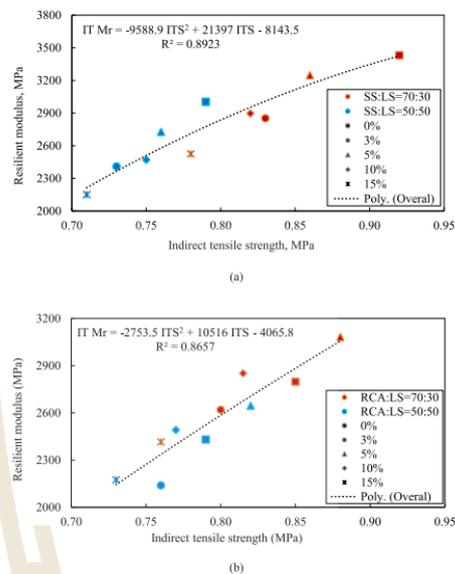
Fig. 11. Relationship between ITS and IT Mr of SS:LS (a) and RCA:LS (b) samples at different r/c ratios.
