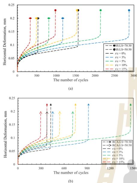
**Fig. 7.** Relationship between the number of cycles and horizontal deformation under fatigue test at 70% stress level: (a) cement- and cement-NRL stabilized SS:LS blends, (b) cement- and cement-NRL stabilized RCA:LS blends at different r/c ratios.
