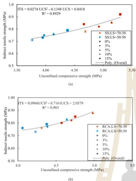
Fig. 10. Relationship between UCS and ITS of SS:LS (a) and RCA:LS (b) samples at different r/c ratios.
