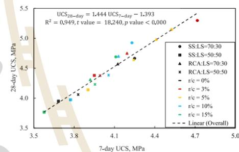
Fig. 7. Relationship between 7-day and 28-day UCS of cement-NRL stabilized SS:LS and RCA:LS samples at different  $r/c$  ratios.
