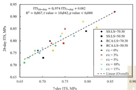
Fig. 8. Relationship between 7-day and 28-day ITS of cement-NRL stabilized SS:LS and RCA:LS samples at different  $r/c$  ratios.
