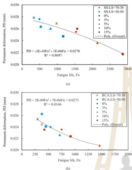
Fig. 13. Relationship between Fatigue life and Permanent deformation of SS:LS (a) and RCA:LS (b) samples at different r/c ratios.
