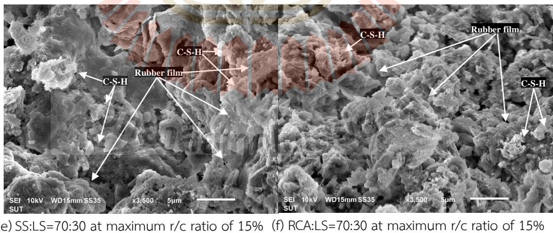
**Figure 3.12** Scanning electron microscope images of cement stabilized and cement-NRL stabilized SS:LS and RCA:LS samples at ages of 28 days.
