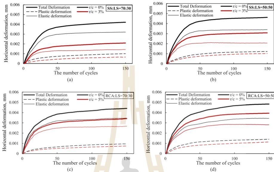
Fig. 5. Relationship between horizontal deformations and the number of cycles under repeated-load at 30 % stress level of cement- and cement-NRL stabilized SS/RCA:LS blends at optimum  $r/c$  ratio: (a) SS:LS = 70:30, SS:LS = 50:50, (c) RCA:LS = 70:30, and (d) RCA:LS = 50:50.
