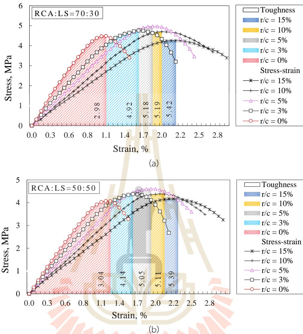
**Figure 3.7** Stress-strain curves of cement and cement-NRL stabilized RCA:LS samples: (a) RCA:LS=70:30 and (b) RCA:LS=50:50.
