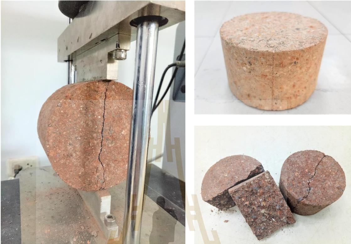
Figure 3.3 Photograph of ITS samples.
